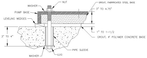
Figure 4-1: Anchor Bolt configuration
