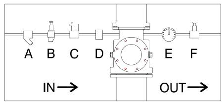
Figure 5-2: Water Flush System
